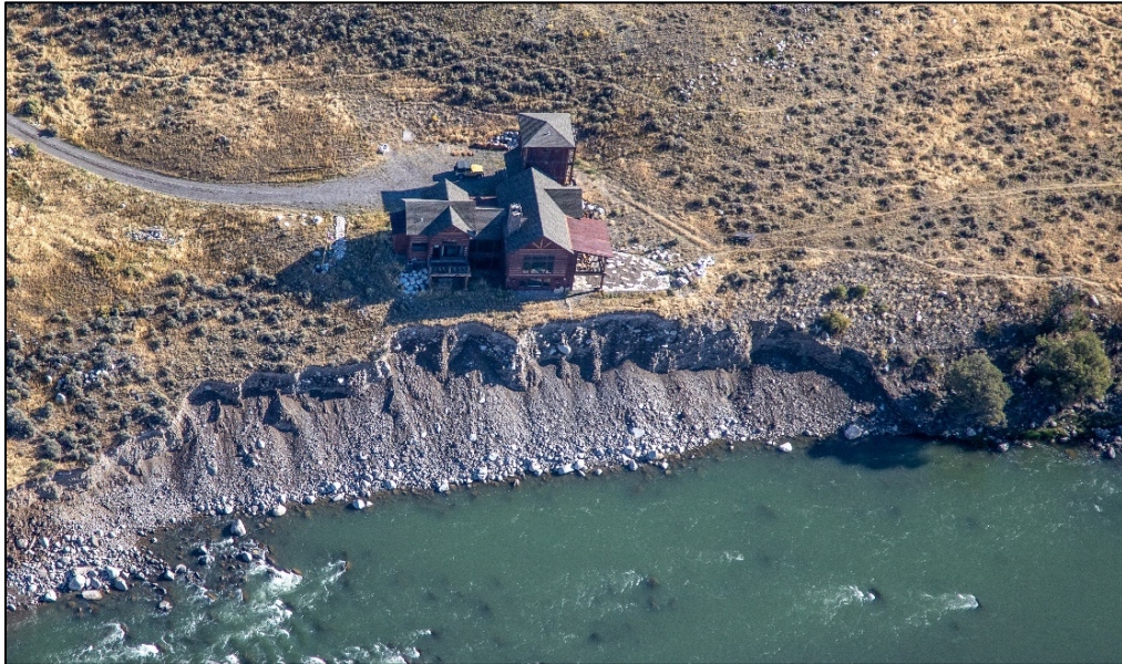
Figure 71. Example high terrace erosion threatening home on upper Yellowstone River, June 2022 (Kestrel Aerial Services).
