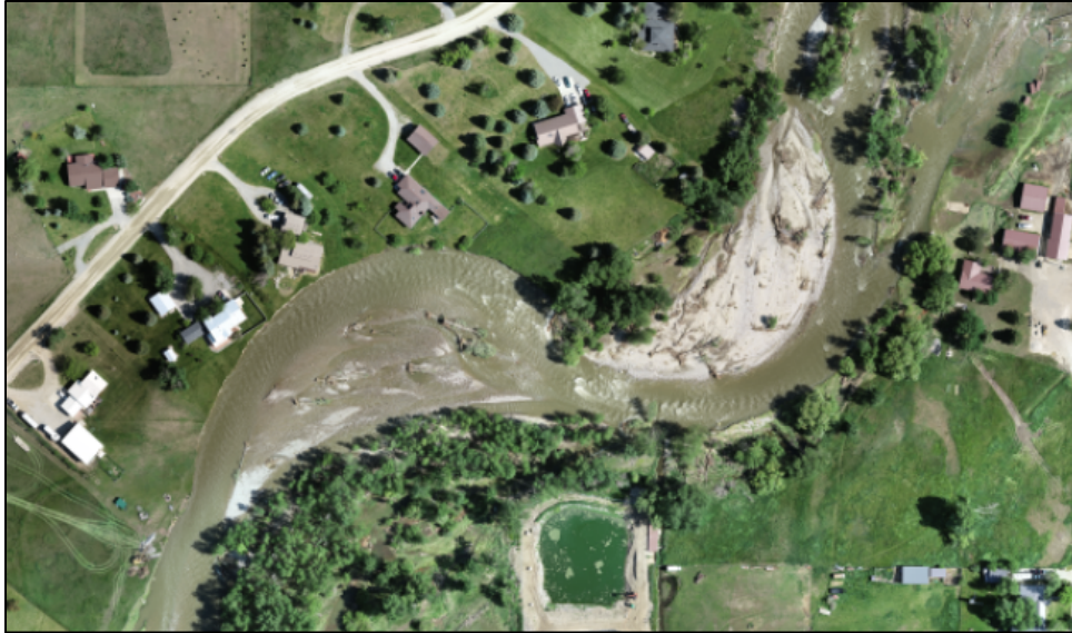
Figure 65. Erosion intensity visible at site shown in Figure 64 during the flood event; the channel flowing against the homes was diverted with a dike to the south, reducing the property threat (see Figure 64). The berm has since been removed.
